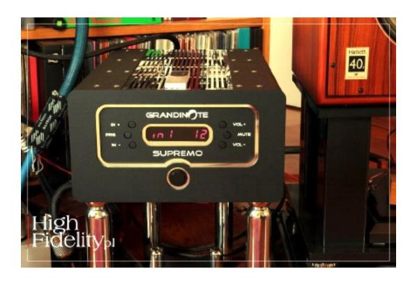
The stand consists of a steel platform, which the aforementioned pins are screwed onto, which act as supports for the amplifier, and low feet. In the pins, semicircular recesses are milled, into which also semicircular, feet fit. It is a simpler version of the bearing, an anti-vibration element that is found in the products of FINITE ELEMENTE, FRANZ AUDIO ACCESSORIES (PL), STACORE or AVATAR AUDIO (PL).
