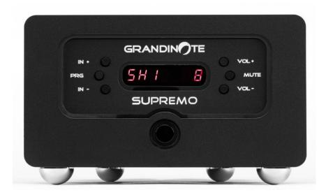
The amplifier works in class A, without feedback and with direct coupling of stages, without the use of capacitors. Yet, it was possible to obtain very high damping factor of more than 230, which translates to a very good control over the speakers, as well as a wide frequency response: from 1.5 Hz to 350 kHz. It is a dual mono amplifier and fully balanced one; inside there are four identical amplifiers, two per channel, one for each half of the balanced signal.
