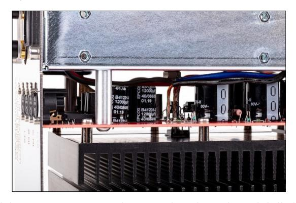
And there are two output transistors per channel, one for each half of the balanced signal, and are bolted to the four large heat sinks in the center. The amplifier gets very hot, so it is worth leaving a lot of free space above and below it. The device works in class A, in a balanced, i.e. push-pull, circuit. The PCBs show separate power circuits, including rectifiers, for each branch of the circuit - so we have here, as I said, four identical amplifiers.
