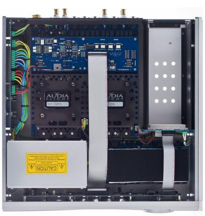
Unlike its predecessor, the Strumento n°1 mk2 does not require a ventilator despite the amplifier stages operating in Class A mode.
