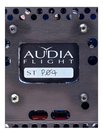
The circuit boards are shielded by these plates; the drill holes allow for the required air circulation.
