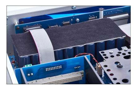
The filter capacitors are mechanically soothed. The plate is intended to also take effect against electromagnetic interference.
