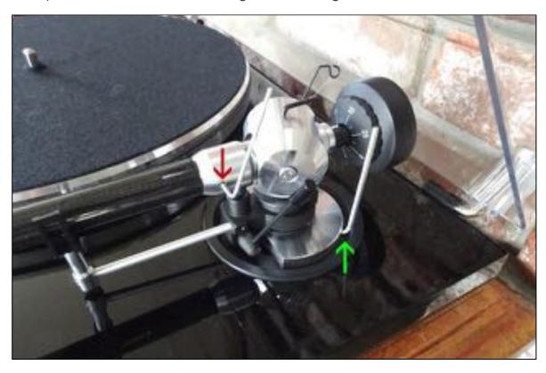
The VTA, when adjusted, will have the distance between the tonearm and the surface of the LP the same for the entire length of the tonearm.
