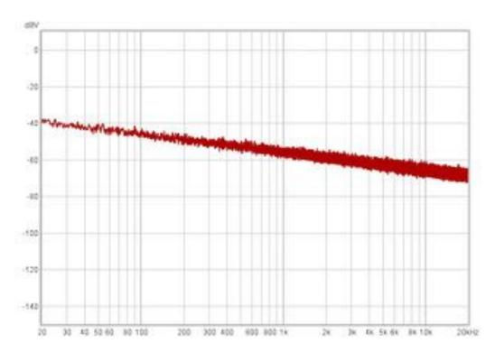
The rumble test is shown below. I used a silent groove (groove on the LP with no signal). The principal rumble is at about 13 Hz.
