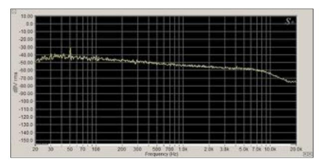
Taking a look at pink noise fed from the sound card's output back to the input (no turntable in the circuit), you can see the straight spectrum with a constant slope.
