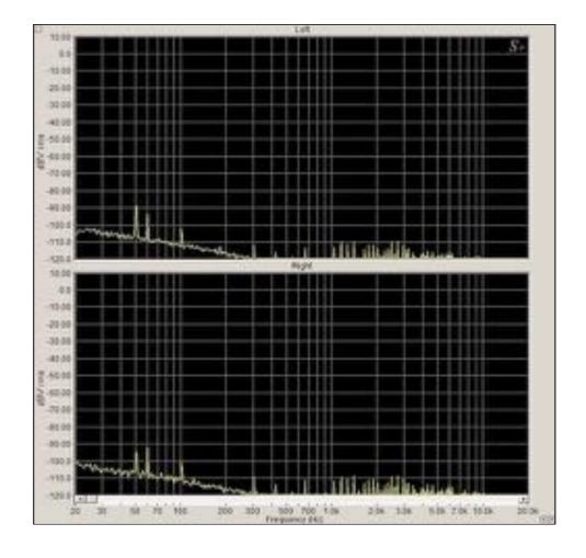
A 1 kHz sine wave test shows THD at 0.67% in the left channel and 0.52% in the right. The largest harmonic is second-ordered, and that is characteristic of vinyl. It gives the listener a warm sound that is very pleasant. The noise peaks have been amplified.
