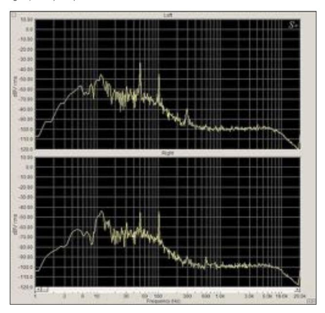
The rumble filter on the phono preamplifier can be used to reduce this, as shown below. The 13 Hz rumble is gone. It did not bother me because my speakers do not respond that low. But it's probably a good idea to use the filter to reduce the amount of amplifier energy that is otherwise wasted.
