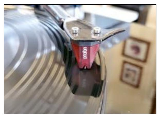
I used a tracking force gauge that I bought on Amazon for about \$13. I set the tracking force at 1.84 gm.
