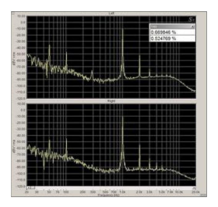
If we zoom in so that we can accurately measure the actual frequency, it is 992 Hz at 33-1/3 RPM. This is an 0.8% error which is more than the spec of  $\pm$  0.15%, but it is still not an audible error. The two side peaks next to the 1 kHz peak are probably Intermodulation Distortion (IM) peaks from interaction with one of the large noise peaks at either 50 Hz or 60 Hz.
