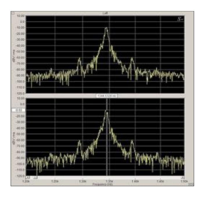
For a cross-talk measurement, I used a 1 kHz sine wave in the left channel. It read -10 dBV. In the right channel, a cross-talk peak showed up at -45 dBV, which represents 35 dBV difference, so that is the channel separation (35 dBV).
