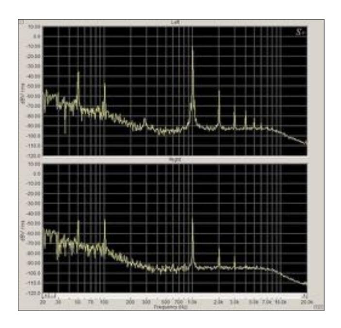
The wow & flutter test result is shown below. A sine wave of 3,150 Hz is used. It displays at 3,124 Hz which, again, shows the speed error. There does not appear to be any flutter. The two side peaks at 3,070 Hz and 3,170 Hz are, in my opinion, Intermodulation Distortion peaks, not flutter.
