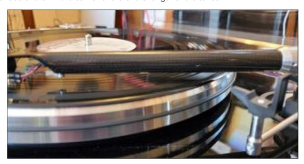
The Azimuth adjustment is used to set the cartridge so that the distance between the left bottom of the cartridge to the left of the needle and the surface of the LP, as well as the distance between the right bottom of the cartridge to the right of the needle and the surface of the LP, are equal.
