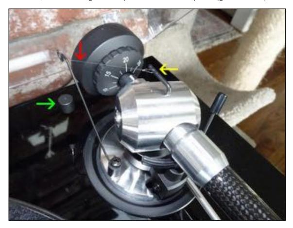
For a tracking force of 1.8 gm, the anti-skate thread is attached to the middle notch on the spindle, pointed out by the yellow arrow below.
