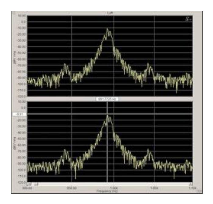
At 45 RPM, a 1 kHz sine wave test track that was recorded at 33-1/3 RPM should be at 1,350 Hz. Here, it is at 1,345 Hz which an 0.37% error. This is larger than the  $\pm$  0.13% spec for 45 RPM. Again, though, this is inaudible. A more accurate speed is one of the things that you pay for in more expensive turntables. In some cases, the speed is actually adjustable for both 33-1/3 RPM and 45 RPM.
