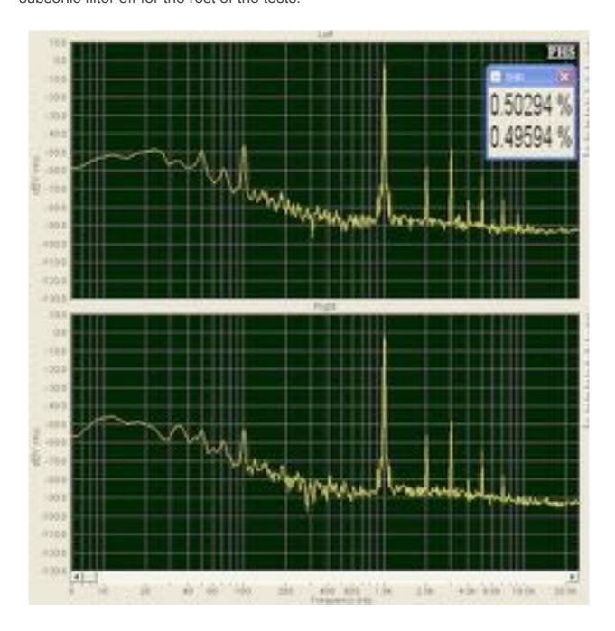
Using a 300 Hz sine wave recorded at + 15 dB, the E.A.T. Jo No 5 had no problems tracking the groove. In this case, the second-ordered harmonic was the largest.
