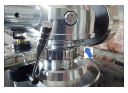
When playing an LP, there is a tendency for the stylus to move towards the center spindle because the grooves near the center are rotating at a lower linear velocity than grooves near the outer edge (the inner grooves are smaller diameter). This is what the anti-skate mechanism corrects.
