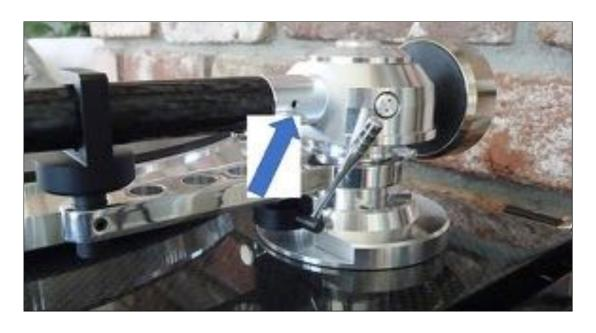
When the screw is loose, you rotate the tonearm until the cartridge cantilever is vertical when resting on an LP. Note: raise the tonearm with one hand and rotate it with the other hand. Do not rotate the tonearm while the stylus is resting on the LP. Once it is vertical, tighten the hex screw (with the tonearm raised). The photo below shows the stylus and cantilever vertical to the surface of the LP.
