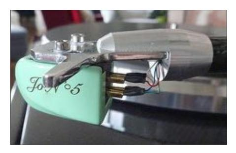
When attaching the cartridge, you don't allow it to rest on the platter since the counterweight has not been attached yet. Leave it in the tonearm rest.
