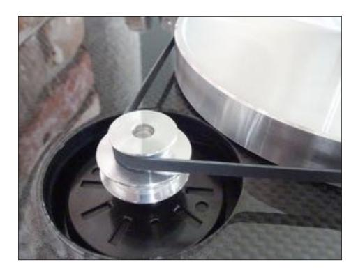
After choosing a platter speed with the belt placement, put the main platter on top of the sub-platter.
