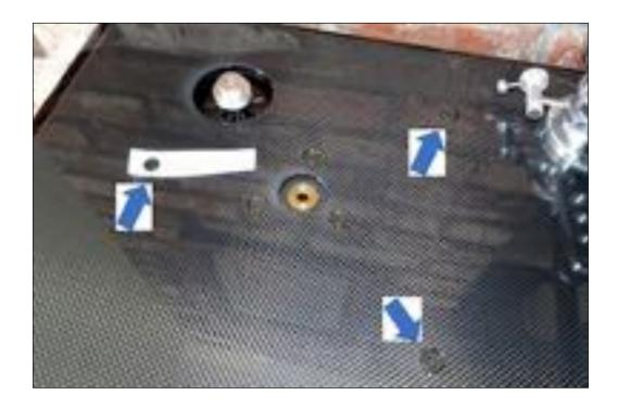
Mount the sub-platter and then attach the rubber belt to one of the motor pulleys and around the perimeter of the sub-platter.
