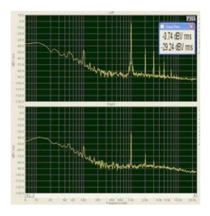
Here is a spectrum with nothing playing (everything connected and powered on, but the stylus in the arm rest, not in a groove). It shows a low frequency noise range at 100 Hz and below, about 30 dB lower than what it is when a track is played. This is surface noise.
