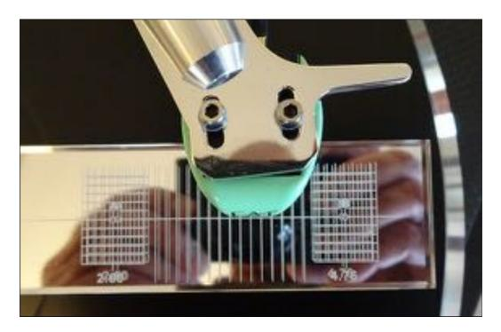
The **Azimuth** refers to having the cartridge not tilted to the left or right, i.e., when looking at the front of the cartridge, not having the left side closer or farther from the surface of the LP than the right side, and more specifically, the cantilever is vertical. To do this on the C-Major turntable, you loosen a hex screw on the side of the tonearm, as shown below by the arrow.
