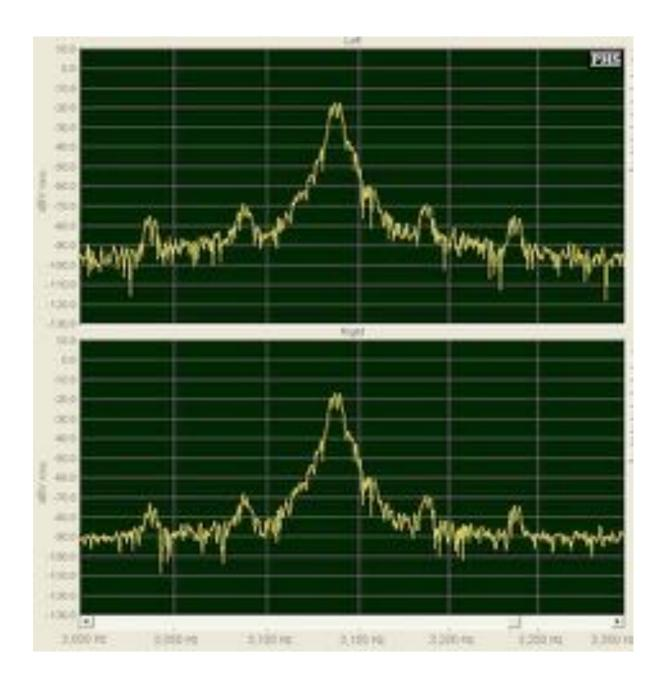
At 45 RPM, there was also a slight speed variation (the 3,150 Hz test signal peak should be at 4,253 Hz because it is being played at 45 RPM). Because this happened at both speeds, I would suggest it is caused by a wall voltage lower than 120 V, which would lower the output voltage of the motor power supply. There appears to be less Wow & Flutter at 45 RPM than at 33-1/3 RPM.
