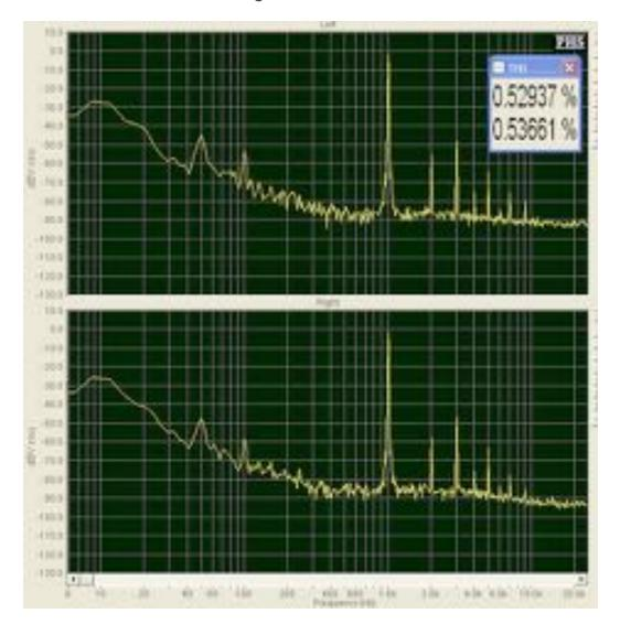
I turned on the subsonic filter for this spectrum (below), which is also a 1 kHz sine wave at 0 dBu. The frequencies at 20 Hz and lower are rolled off. So, I left the subsonic filter off for the rest of the tests.
