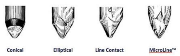
The surface area that contacts the groove is shown in the figure below. You can see that the Line Contact types have about 100  $\mu$ m2 surface area contact compared to about 35  $\mu$ m2 of the spherical and elliptical styli from decades ago (see the second row from the bottom, Row E). This means that modern phono cartridges produce a much more accurate sound from the vinyl groove than they used to do. (Diagram copyright Audio-Technica)
