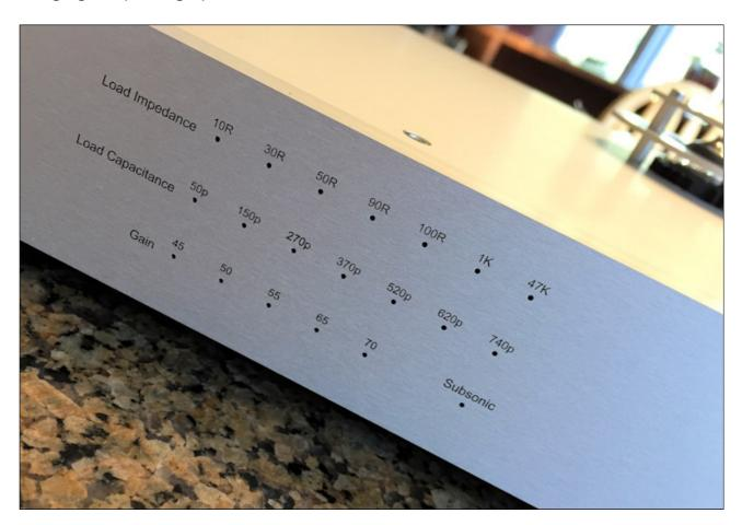
What the EAT E-Glo S provides is input impedance for MC cartridges at 10,25,50,75,100,1000, 47K Ohm and gain settings at 45,50,55,65,70 dB, a few less clicks than the E-Glo. While the MM gain is 45 dB. Each selection is illuminated with a small LED indicator on the faceplate but you may have to squint a little bit to see them.
