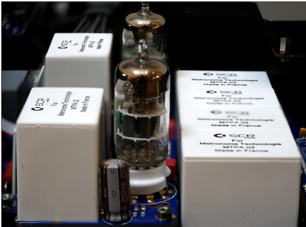
.. finishing up with the joint army/navy 6922 in their ceramic sockets and French-made SCR capacitors. The transistor outputs use 4 x class A-biased Texas Instruments OPA 604 opamps.
