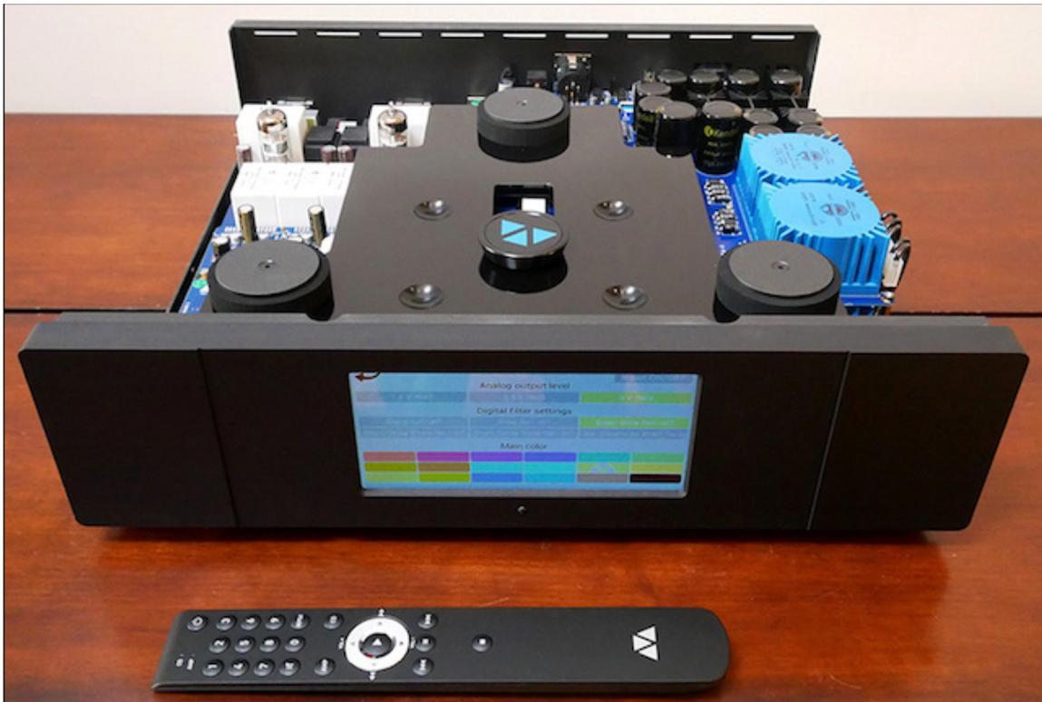
The first thing to strike the eye would surely be the shiny black 'helipad' for the discs. It's supported on three massive rubberized pillars for effective decoupling from what the AQWO sits on.
