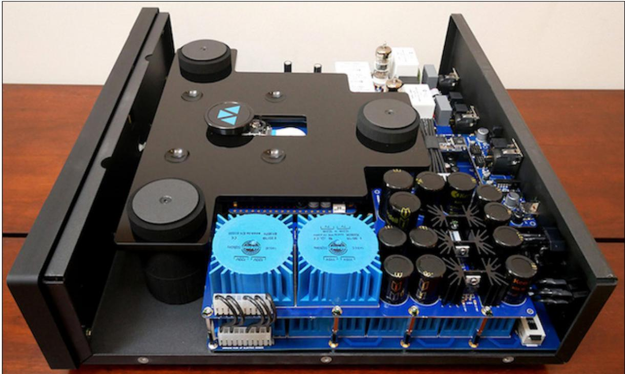
Here's a closer look at the tube buffer's triodes and adjacent D/A converter board
