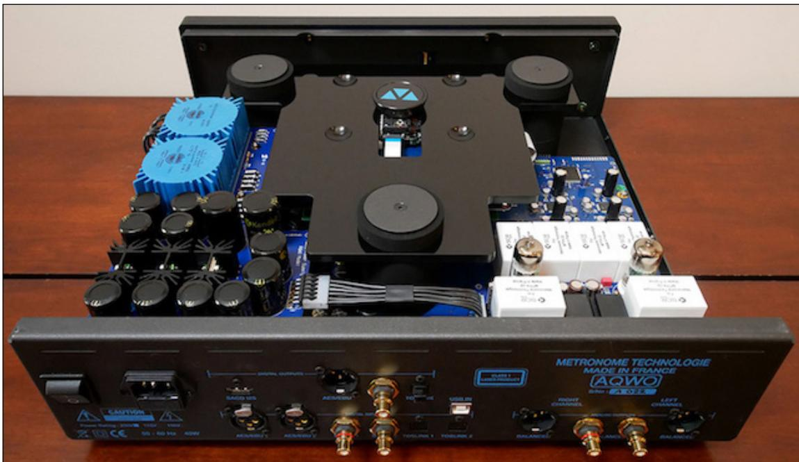
The next thing to say hello were two small valves surrounded by Métronome-branded boxy white caps and two tiny transformers; and stout filter capacitance across the aisle with heat-sinked voltage regulators and two small fully encapsulated blue toroidal transformers.
