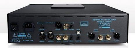
THE USB INPUT WILL ACCEPT FORMATS UP TO DSD512, WHILE THE OTHER INPUTS ACCEPT UP TO 768KHZ/32-BIT PCM IN ADDITION TO DSD UP TO DSD512/8×DSD.
