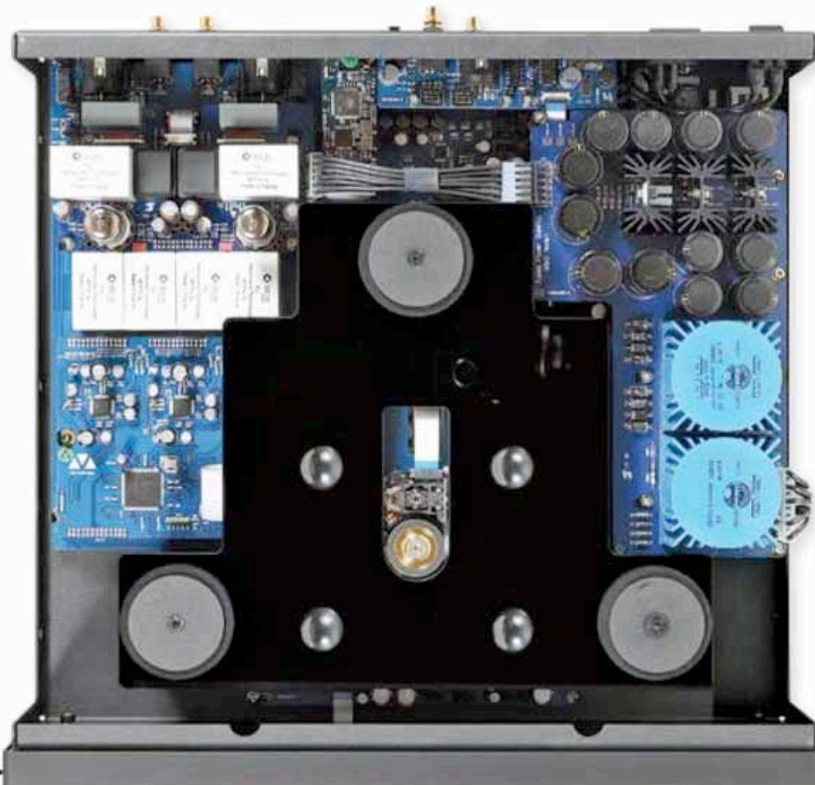
RIGHT: Métronome's blue encapsulated Talema transformers feed PSUs [top right] for the tube [top left] and solid-state analogue outputs. Two AK4497 DACs [left] support both CD/SACD via a 'floating' top-loading transport
