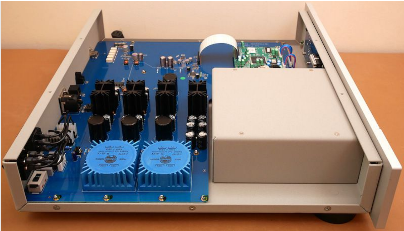
... gets 2 x 7.5VA transformers plus the same four voltage regulators with finned heat sinks as the CDP/DAC.
