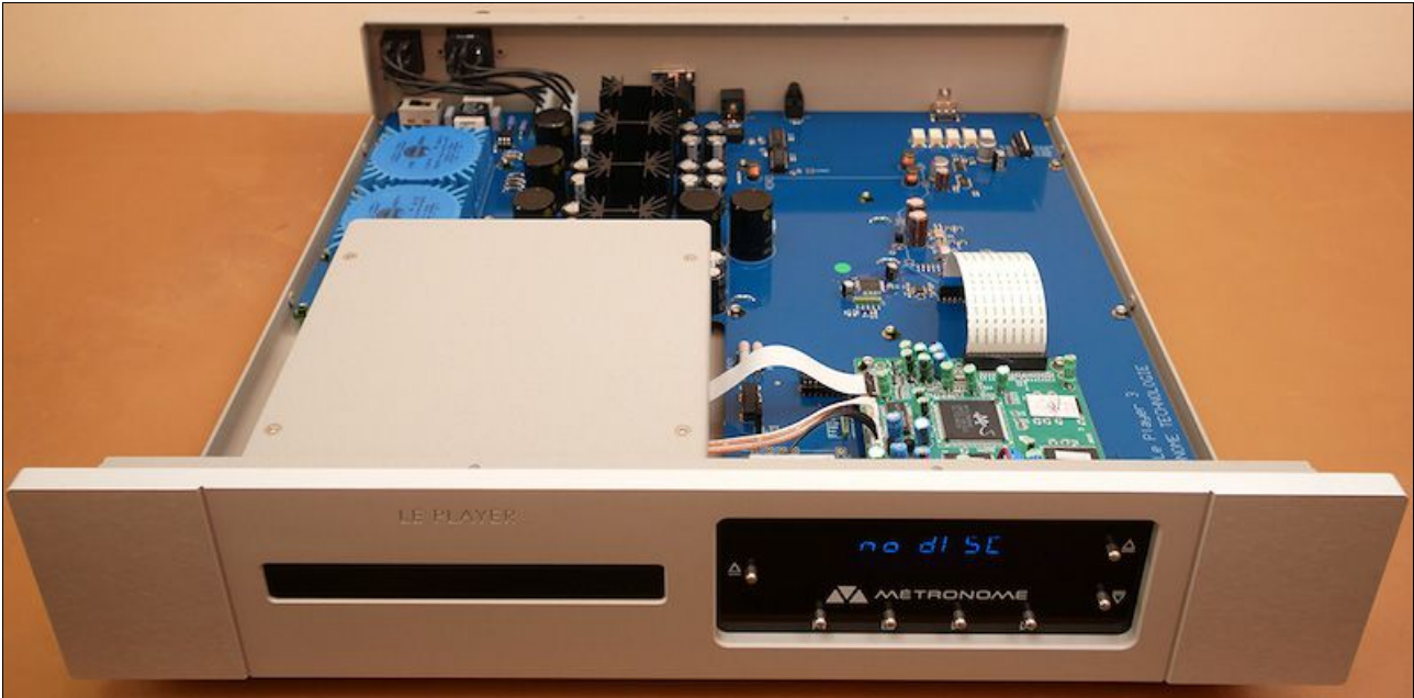
... gets 2 x 7.5VA transformers plus the same four voltage regulators with finned heat sinks as the CDP/DAC.
