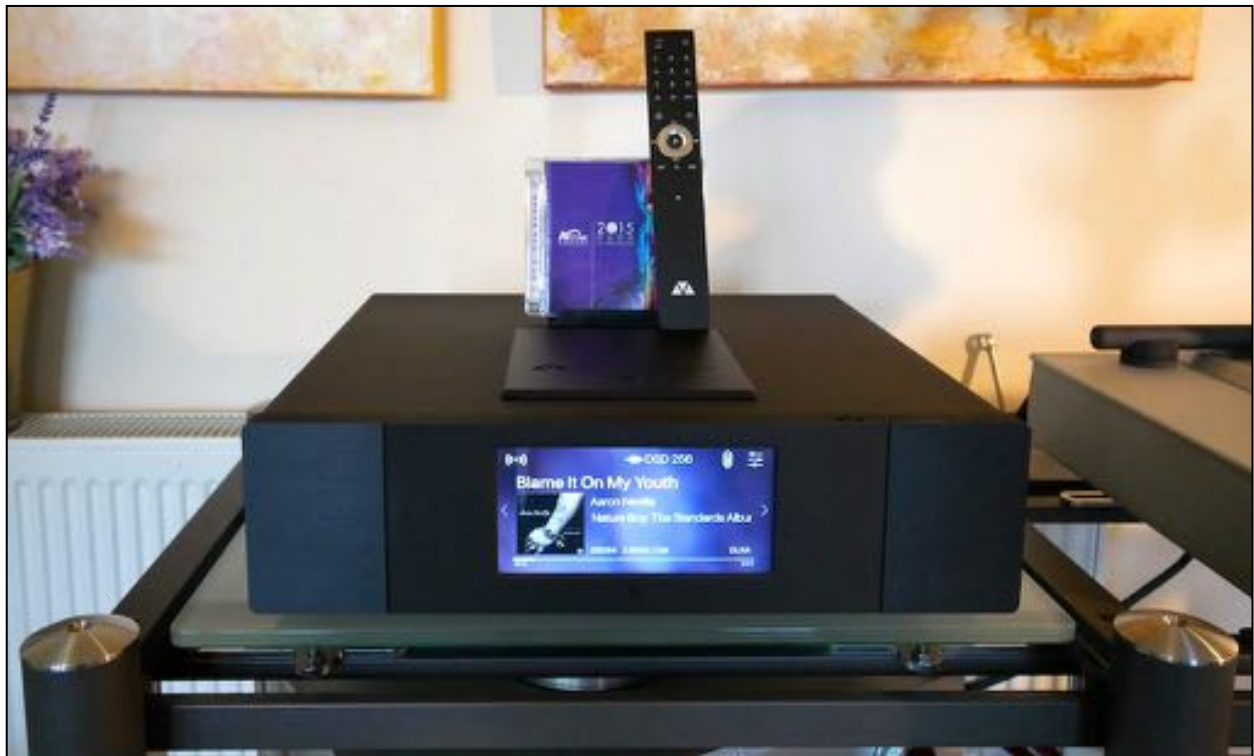
Right-click image to open at full size in new tab. The display shows streaming mode, tube outputs engaged, DSD64 signal coming in via DLNA, upsampler for I2S output set to DSD256.
