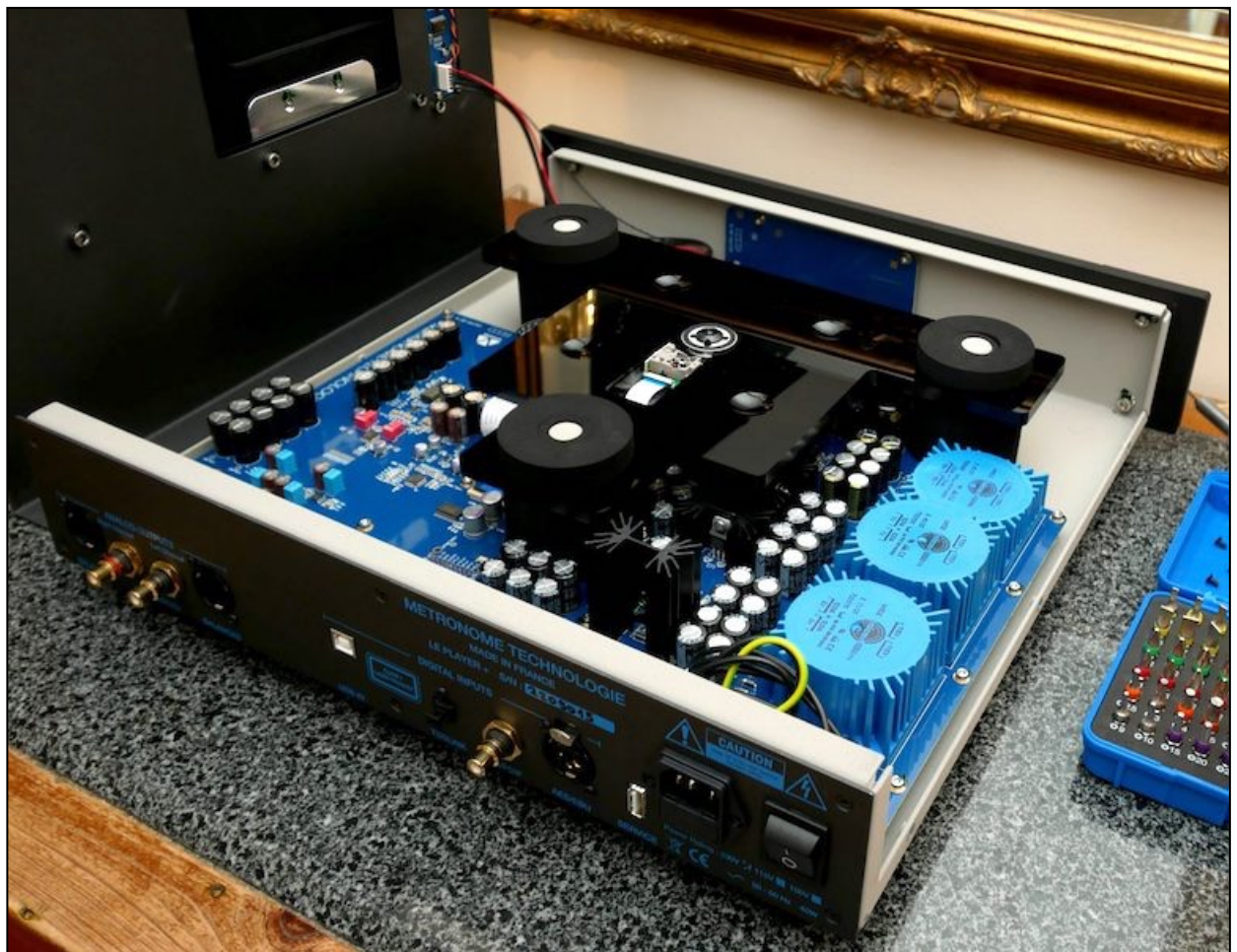
Here we see the converter chip and OXCO clock.
