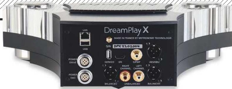
**ABOVE:** The 'fully loaded' DreamPlay XC has two PSU inputs, wired/wireless network ins, a USB-A port for external drives (and one for service) plus digital outs on HDMI (I<sup>2</sup>S), XLR (AES/EBU) and coax (S/PDIF). Fixed/variable analogue outs are on RCAs and XLRs
