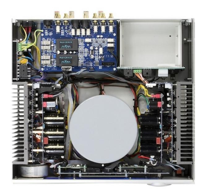
The FLS9 is quite customisable. For example, you can increase or decrease the gain of each individual input by +/- 6dB to equalise volume levels between different inputs. You can even add dither – a low-level hiss that helps mask digital artefacts that can lead to quantisation distortion. Classy!
