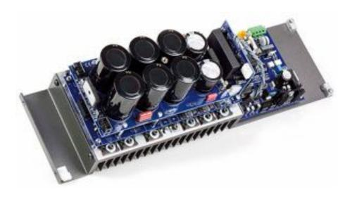
Instead of six pairs of bipolar transistors handling both the positive and negative-going sides of that amp, the FLS 9 has six pairs of very capable MJL1302A/3281A bipolars from ON Semiconductor forming each complementary channel. Power output is considerable and also very load tolerant thanks to the stiffly-regulated PSU comprising a screened 1kW toroidal transformer and  $6x10,000\mu$ F reservoir capacitors per side. **PM**
