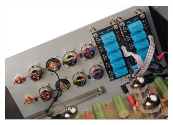
Finest construction with meticulously kept cabling. The inputs are switched cleanly via relays.
