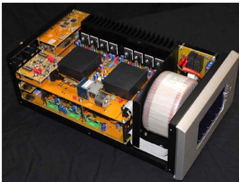
Inside the amp show a well laid-out multilevel construction
