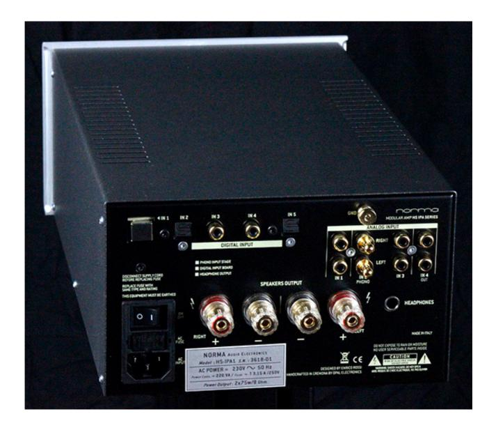
The connectors are all high quality and gold plated. There are four pairs of analogue RCA inputs, one pair of which connects to the optional phono stage, as well as USB, Toslink and S/PDIF for the optional DAC. The headphone socket is also on the rear panel - the matching amplifier is another optional extra. The Norma remote control is a chunky aluminium lump with a large array of buttons to cover every function. The buttons are a little small but it works perfectly well.
