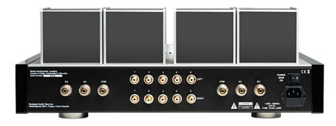
At the back are five pairs of RCA phono connectors, two sets of multi-way speaker binding posts with both 40hm and 80hm values, a mains socket and the on/off rocker working in conjunction with a standby toggle on the front of the amp and the power button on the remote. At the front, blue LEDs show the selected source. To their right, next to the remote sensor, an LED shows power-on, flickering during the 40-second muted warm-up period.
