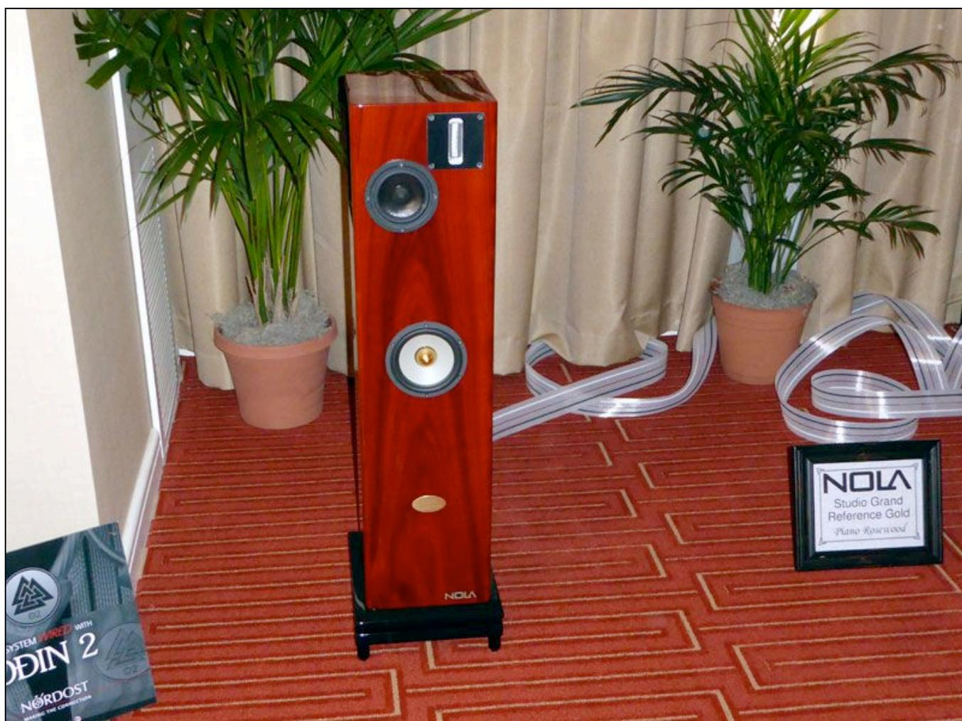
Nola's new Studio Grand Reference Gold (\$19,800/pair) has all of the features of the larger speakers in the Studio Grand series, such as the alnico magnesium woofer with gold phase plug and alnico open-baffle midrange -- all in a compact, room-friendly footprint.
